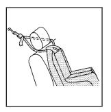
If the position you are using has a fixed or adjustable headrest or head restraint and you are using a dual tether, route the tether around the headrest or head restraint.
